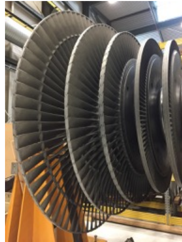
Photo 76: Rotor undergoing major maintenance
