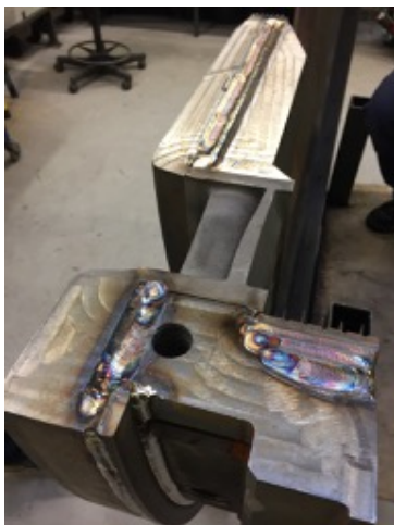
Photo 81: Turbine parts welding
