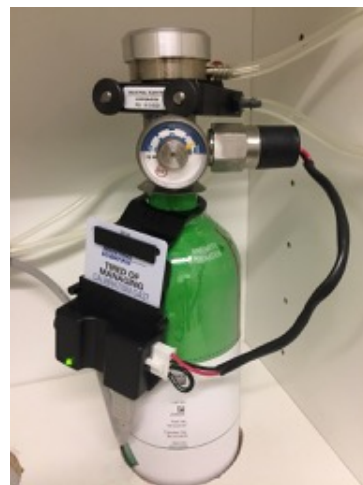
Photo 86: Personal H 2 S meter self-calibration
